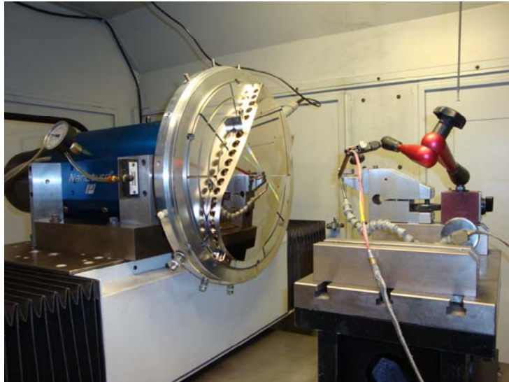
Figure 4: Diamond turning of the main mirror
